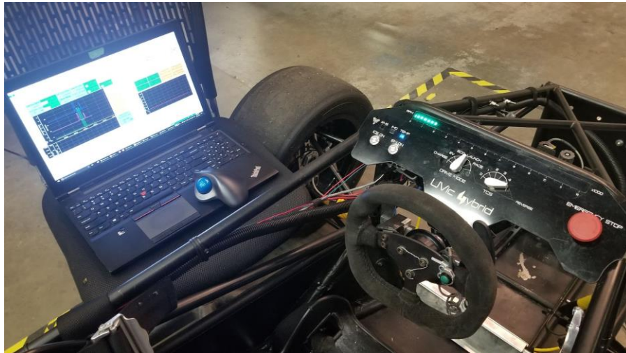
Figure 9: Calibrating the sensor values for the accelerator and brake pedal
