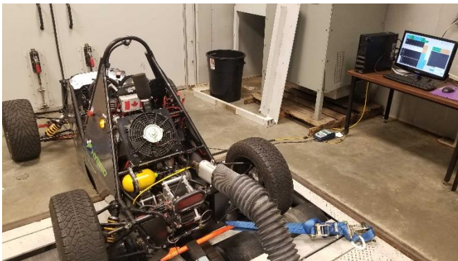
Figure 7: Dyno and track testing the vehicle. It is worth noting the dynamometer hasn't been fixed at the time of testing and we were only using the rollers on a moving surface (no load). Therefore, data regarding torque and horsepower from the dyno can't be measured.
