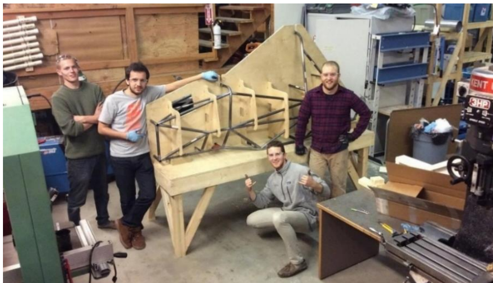
Figure 3: Helping the team mount the frame to the Jig for welding
