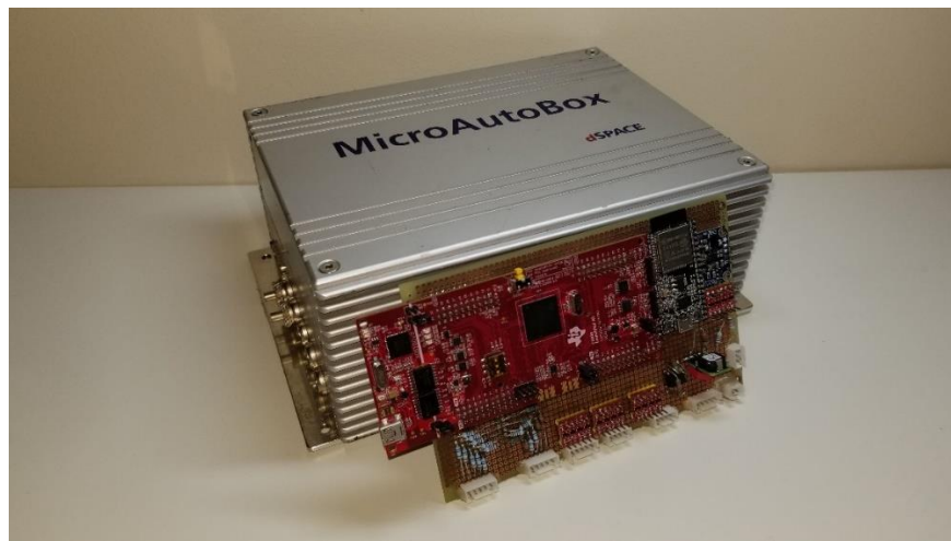
Figure 5: A prototype of the new vehicle supervisory controller next to the MicroAutoBox II (MABx), which it replaces. Compared to the MABx, the new controller is lighter and smaller making packaging easier. It also includes other features like IMU, GPS, and Wifi communication.
