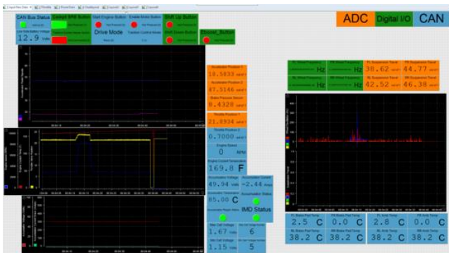
Figure 8: Examples the layouts I created in ControlDesk to monitor and record data (temperature sensors are not calibrated so they are sending wrong values)
